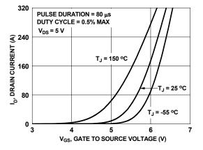
Figure 5. Transfer Characteristics
