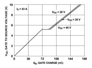
Figure 7. Gate Charge Characteristics
