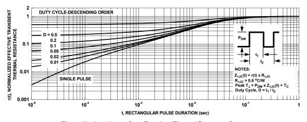
Figure 13. Junction-to-Case Transient Thermal Response Curve
