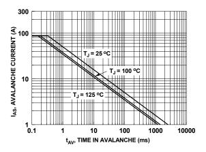
Figure 9. Unclamped Inductive Switching Capability
