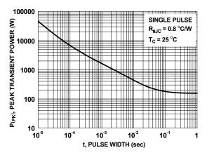
Figure 12. Single Pulse Maximum Power Dissipation
