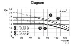
Derating diagram (conductor cross section: 4.0 mm<sup>2</sup>)
