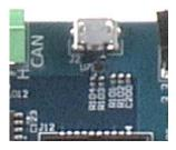
The Synergy S7G2 MCU features independent USB 2.0 Host and USB 2.0 Device (or "function") ports; the Host port capable of High Speed 480mbps data rates, the Device port limited to Full Speed 12mbps.
