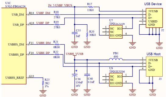
The ports are connected to the MCU as follows:
