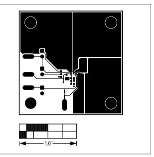
Figure 3. MAX15062C 12V EV Kit PCB Layout—Component Side
