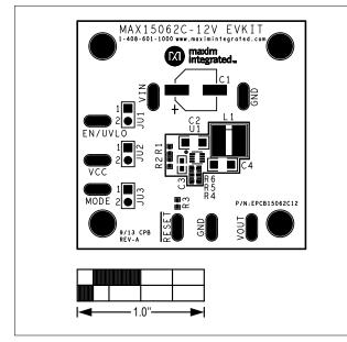
Figure 2. MAX15062C 12V EV Kit Component Placement Guide—Component Side
