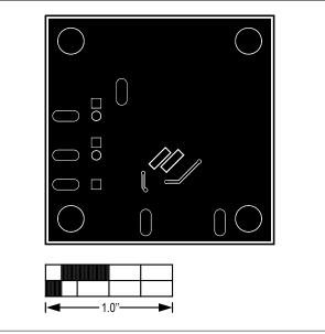
Figure 4. MAX15062C 12V EV Kit PCB Layout—Solder Side
