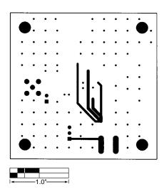
Figure 6. MAX2620 EV Kit PC Board Layout—Power Plane
