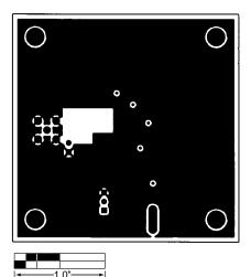
Figure 5. MAX2620 EV Kit PC Board Layout—Ground Plane
