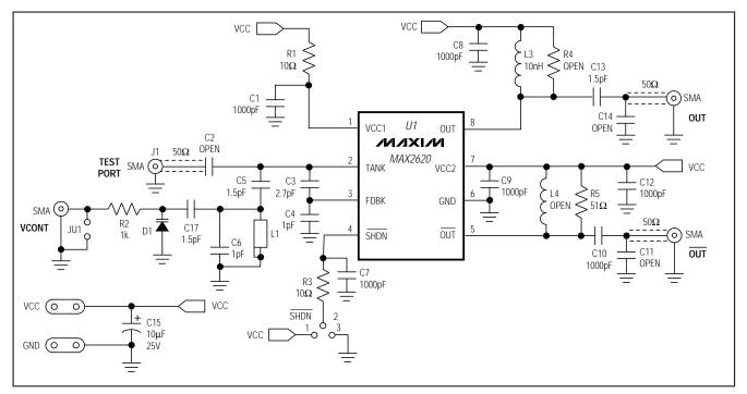
Figure 1. MAX2620 EV Kit Schematic
