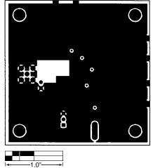
Figure 2. MAX2620 EV Kit Component Placement Guide— Top Silk Screen
