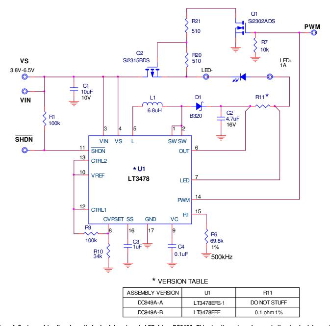
Figure 4. Customer friendly schematic for buck-boost mode LED driver DC949A. This circuit requires changes to the standard demo circuit such as addition of new components and a trace cut on the top-side of the board between the drain of Q1 and the LED- terminal.
