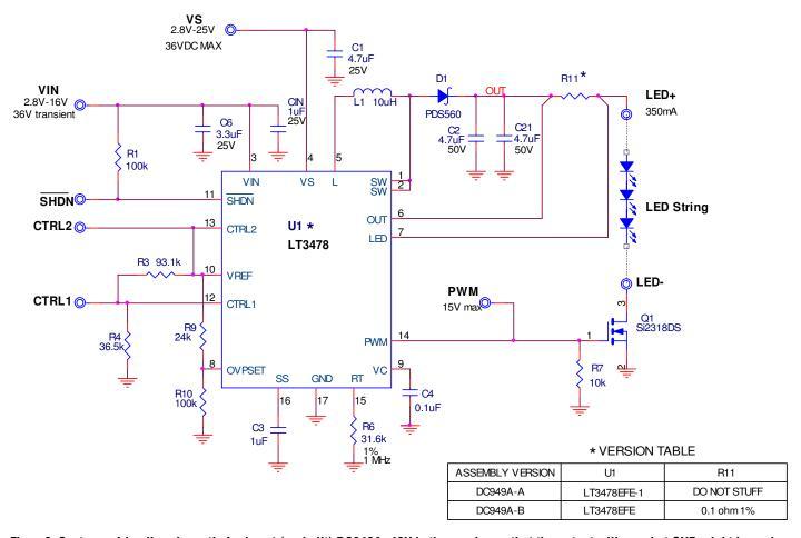
Figure 3. Customer friendly schematic for boost (as-built) DC949A. 40V is the maximum that the output will see, but OVP might be as low as 36V without any adjustments.
