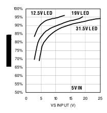
Figure 2. DC949A-A efficiency
