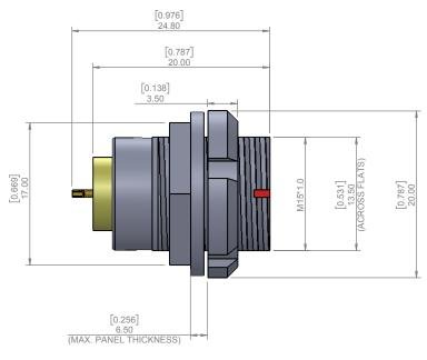
**CHARACTERISSTICS MATERIALS** SHELL: BRASS SHELL PLATING: NICKEL NUT: BRASS NUT PLATING: NICKEL LATCH SLEEVE: BRASS
