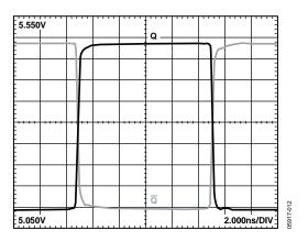
Figure 13. Output Waveform at  $V_{CC} = 5.5 V$
