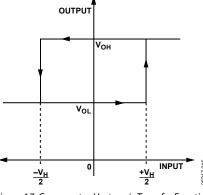
Figure 17. Comparator Hysteresis Transfer Function
