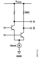
Figure 14. Simplified Schematic Diagram of CML-Compatible Output Stage
