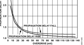
Figure 10. Propagation Delay vs. Input Overdrive
