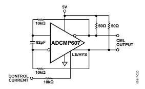
Figure 21. Current-Controlled Oscillator on the ADCMP607
