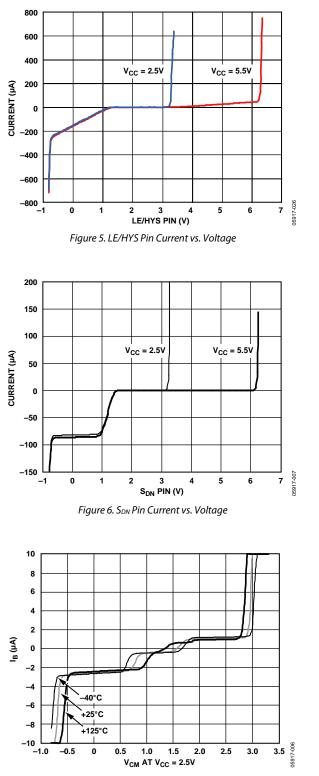
Figure 7. Input Bias Current vs. Input Common-Mode Voltage
