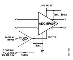
Figure 24. Hysteresis Adjustment with Latch on the ADCMP607
