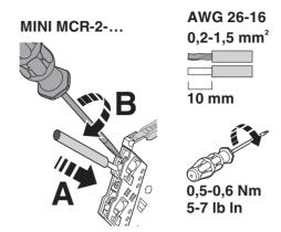
Figure 4 Screw connection
