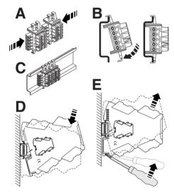
Figure 3 Mounting and removing
