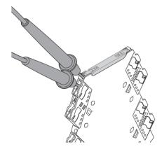
Figure 6 Test disconnect terminal block
