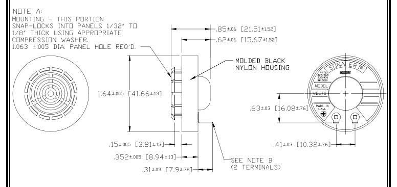
NOTE B: TERMINALS - .016 BRASS, HOT TIN FINISH WITH .076 WIRE HOLE. TERMINAL WILL ACCEPT STANDARD 1/8" QUICK CONNECT
