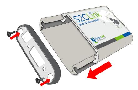
3.1.5 Step 5: Insert the PCB assembly into the enclosure. The side of the PCB with the DB9 should be inserted first. Make sure it is not inserted upside down. Be sure to copy the MEID/IMEI/SIM ID from the Skywire so it is easily accessible after the device has been assembled.
