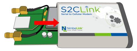
3.1.6 Step 6: Attach the RF face plate to the enclosure. Make sure that the SIM extender is aligned to the slot in the middle of the face plate for the SIM card.
