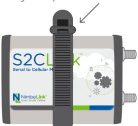
Tighten strap around device.
