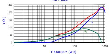
AGILENT E4991A Impedance/Material Analyzer HP 16092A-Test Fixture REF #4101
