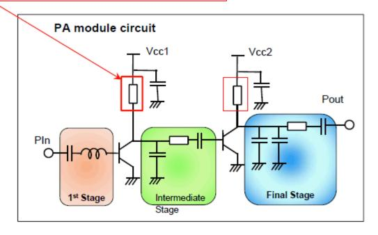
Target use as choke/isolation inductor in RF amp due to high DC current capabilities
