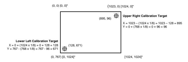
\*The coordinates are in *video* terms, with the origin (0, 0) in the upper left corner of the sensor. Examples from the *controller's* perspective, however, place the origin at the lower left corner of the sensor (numbers in brackets). The controller outputs 0 to 64K on both axes independent of display screen resolution.
