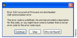
Figure 12. Board Detection Failure
