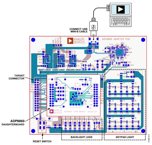
Figure 13. ADP8860 Board Connections
