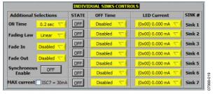
Figure 19. View/Modify Individual Sinks Parameters
