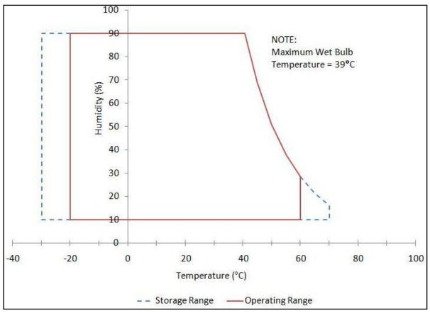
Figure 1 - Operating Temperature and Humidity Range
