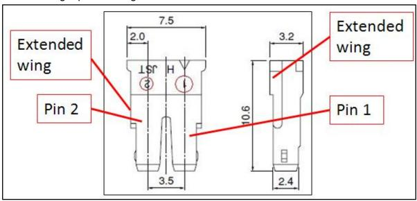
Figure 7 - Backlight Pin Ordering
