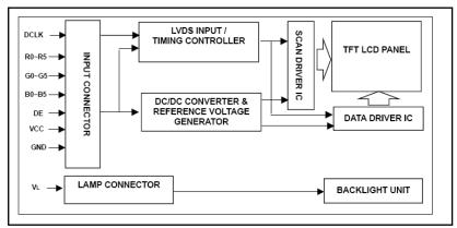
Figure 8 - LCD Block Diagram
