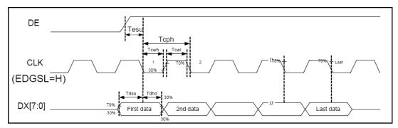
Figure 4 - LCD Interface Waveform
