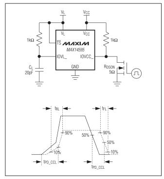
Figure 4. Open-Drain Driving IOVCC\_
