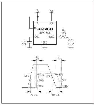
Figure 3. Push-Pull Driving IOVCC\_
