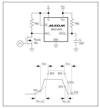
Figure 2. Open-Drain Driving IOVL\_
