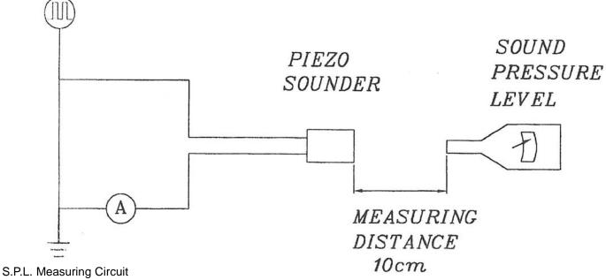
Input Signal: 10 V p-p, 2.0 KHz, Square Wave
