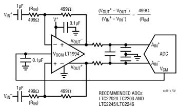
Figure 2. Typical Application for an LT1994
