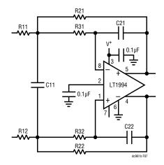
Figure 7. Fully Differential, 2nd Order, Lowpass Filter Design Schematic
