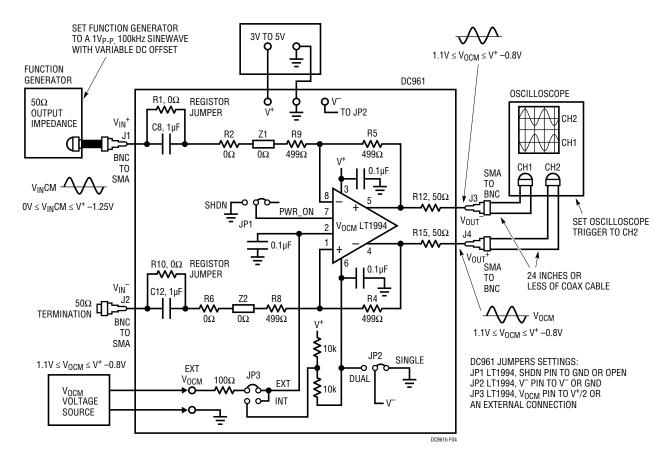
Figure 4. Input and Output Common Mode Quick Test Setup
